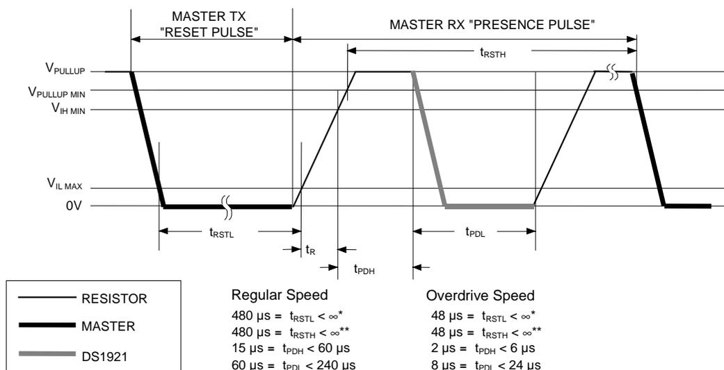
\* In order not to mask interrupt signalling by other devices on the 1-Wire bus,  $t_{RSTL} + t_R$  should always be less than 960  $\mu$ s
