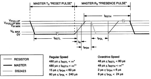
\*IN ORDER NOT TO MASK INTERRUPT SIGNALING BY OTHER DEVICES ON THE 1–WIRE BUS,  $t_{RSTL}$  +t\_R SHOULD ALWAYS BE LESS THAN 960  $\mu s$  \*\*INCLUDES RECOVERY TIME
