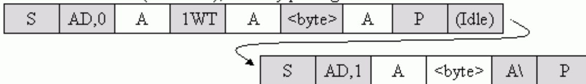
Figure 9. 1-Wire Triplet. Performs a Search ROM function on the 1-Wire line. The idle time is needed for the 1-Wire function to complete. Then access the device in read mode to get the result from the 1-Wire Triplet command.
