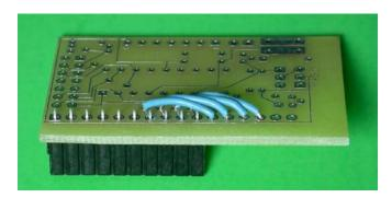
(3) 2x7 (J3) socket or pin header direct to display, inserted on bottom of board, soldered on top side.
