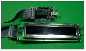
An example of a not so common connection might be this VFD display. While it has a standard 2x7 connection, the female connectors are tiny, accepting a pin similar to those on a solder tail machine pin DIP socket. (see picture on next page)
