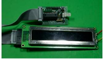
(4) 2x7 (J3) pin header to connect to ribbon cable, inserted on top side, soldered on bottom side. Holding the K107 board with chip writing readable and J3 on the left, J3-1 will be the upper right pin.
