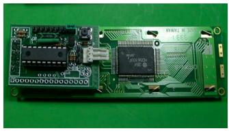
(3) 2x7 (J3) socket or pin header direct to display, inserted on bottom of board, soldered on top side.
