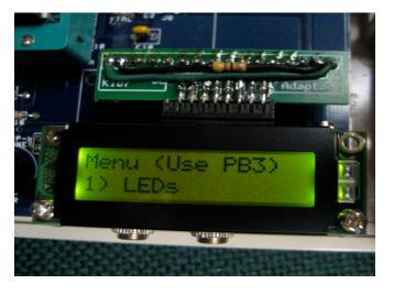
Now clip the 1x16 pin header to 14 pins and insert and solder, pins down solder on top.
