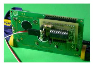
(1) 1x14 or 1x16 (J2), socket header, inserted from bottom of board soldered on top (component) side. Despite the fact that pins 7-10 are usually unused, it is recommended to use a socket (or pin) header with all 14-16 pins as this provides the most rugged mounting rarely requiring anything further to secure the lightweight K107 to the display.
