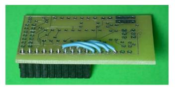
(2) 1x10 (J2) socket header, inserted from the bottom side and soldered on the top. Pins 7, 8, 9, 10 each have an extra hole adjacent to it to allow jumpering to 11, 12, 13, 14 respectively. Some displays shift the pin functions down four positions to the oft unused pins 7-10.
