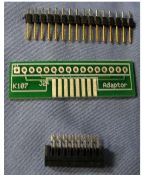
The 16 .100" spaced holes number 1 to 16 left to right, pin 1 having a square pad. Pin 1 of the FFC connector is on the bottom beneath the silk-screened "1" just visible above and right of the "J2" silk-screen. The first FFC pin visible on the top is #2.
