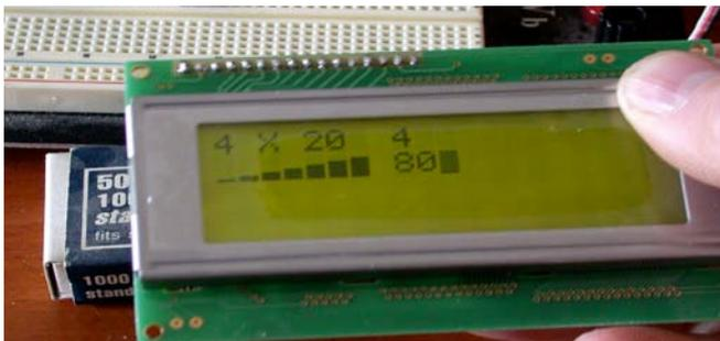
**\*Caution\*** As previously stated, the Anderson chip has a 64 byte buffer. Generally speaking, typical LCD screen displays will rarely tax this limit,
