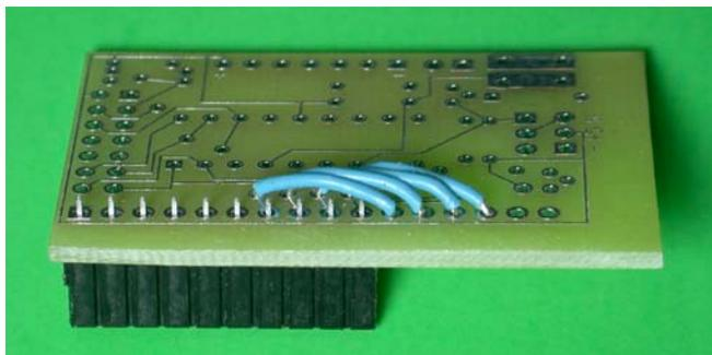
(2) 1x10 (J2) socket header, inserted from the bottom side and soldered on the top. Pins 7, 8, 9, 10 each have an extra hole adjacent to it to allow jumpering to 11, 12, 13, 14 respectively. Some displays shift the pin functions down four positions to the oft unused pins 7-10.
