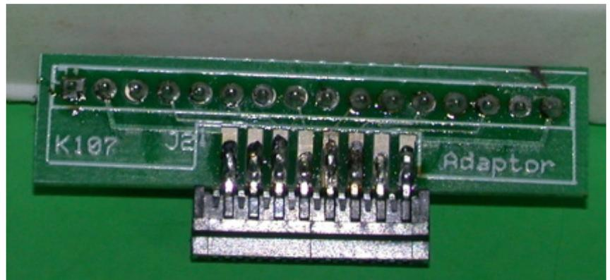
If you mess up the FFC connector and get it aligned wrong, this tip from customer John Brayton may help ... "The method I used to un-solder the connector: I took a very small hypodermic needle, 1.5" long, 29 gauge, and gently inserted it under every tang as I applied heat. Because the solder doesn't stick to stainless steel I was able to work across each side of the connector, slowly and carefully, until it popped off."
