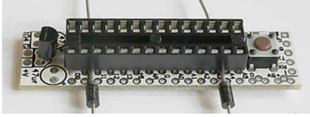
Spacing the socket off the board with some resistor or diode leads will make the pcb labels more legible
