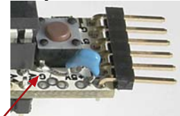
Connect the other lead of the cap to the reset switch pin closest to the Atmega chip.
