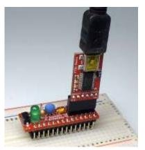
The FTDI adapter *can* power the Ardweeny *and* the other circuitry on the breadboard, if you connect the 'GND' and '+' pins to the rest of the breadboard power rails.
