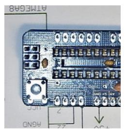
Install the the 6 mm pushbutton reset switch. Hold so the prongs go up and down (not left and right) Center the switch and bend the prongs and solder.
