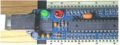
Insert chip, notch on chip aligned with notch on socket.
