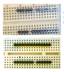
(iDuino v2) Take the four single row pin headers (1x4, 1x6, 1x8, and 1x10) and insert, long side of pin down, them into a breadboard as shown
