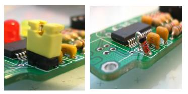
(iDuino v3) provision for diode or jumper to isolate the baord Vcc buss from the FTDI chip Vcc supply. Diode goes in as shown, with band up.
