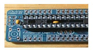
As mentioned on the parts list the Wulfden kit contains two 3M sockets, an 8 pin and a 20 pin (v2/v3) or two 14 pin (v3 only). They can be placed in either order, but have the notch to the left when the board is oriented so you can read the silkscreen. With these sockets C1 (v2) will fit under easily. Make sure you solder every pin.
