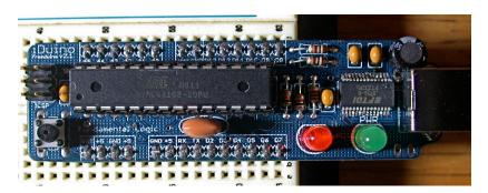
Place the PCB onto the pins and carefully solder, making sure not to heat any one pin for too long. v2 board shown, same instructions for v3
