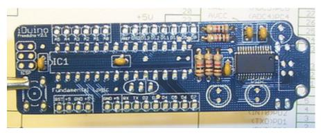
Install the 10 Kohm resistor (brown-blackorange) and the five monolithic 0.1 uF capacitors ("104")
