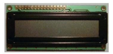
I bought a box of 48 pcs of these 2x16 char LCD modules on eBay. The modules have standard green backlight (with black characters). PCB dimensions are 80x36mm, and the viewable area of the display is 65x14mm.
