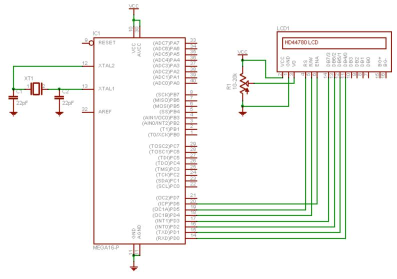
Actually I used the STK500-kit and mounted the LCD module on a bread-board, connected to the PORTD-connector of the STK500. I used a separate 5V power-supply for the LCD, since the backlight can be a little heavy on the power-consumption, and I do not know how much power the STK500 can supply.
